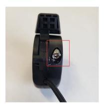
If the lever of the throttle gets stuck, the Scoot Control should not be used anymore. The device needs to be sent back to mo-vis for further investigation.
