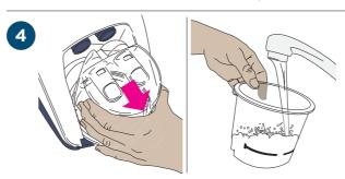
Remove water chamber. Pour out and discard the remaining water. Remove chamber base. Wash the chamber top and base in mild dishwashing detergent then rinse. Soak the chamber in a solution of vinegar (1 part) and water (2 parts) for 10 minutes. Rinse and dry.
