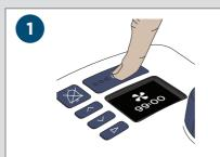
After use, remove your interface. To begin | Rinse the interface in drinking-quality water the 99-minute Drying Mode, press and hold then reconnect to the heated breathing the On/Off button for 3 seconds. To avoid tube whilst still in Drying Mode to dry the burns, do not wear the interface during interface. Drying Mode and do not remove the water chamber until Drying Mode is complete.
