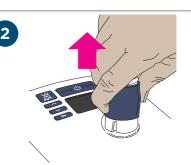
Remove the heated breathing tube and drain any excess condensate.
