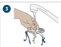
Remove the interface from the heated breathing tube, wash it in warm water with mild dishwashing detergent added, rinse it in drinking-quality water, then reconnect it to the heated breathing tube.
