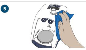
Thoroughly wipe the inside of the heated breathing tube connection port with a clean, low-lint cloth dipped in warm water with mild dishwashing detergent added. Wipe the exterior of the unit with a clean damp (not wet) cloth dipped in warm water with mild dishwashing detergent added.
