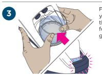
Fit the water chamber onto your device by depressing the finger guard, pushing forward until the finger guard clicks into place.
