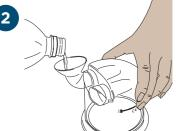
With the aid of the supplied funnel, fill the chamber with enough distilled water for the period of use, but never above the 560 mL maximum water level line.
